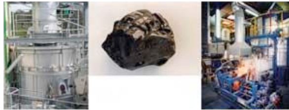
left to right The asbestos vitrification line run by Inertam in Morcenx, France n Cofalit: an inert and non-hazardous vitrified product n The ash melting unit in Cenon, France
